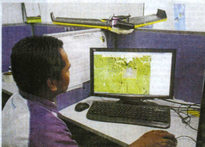
Prepping: Prior to taking off, the team simulates the flight path of the UAV to know if the coverage areas are sufficient to collect data, which would then be analysed to create a meaningful report for clients.
