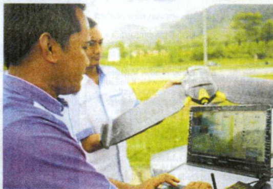
Programmable: The UAV has to be programmed with the flight path, and sometimes needs to be adjusted on the site because of obstruction from both natural and man-made elements, such as wind speed, temperature and also buildings and lamp posts.
